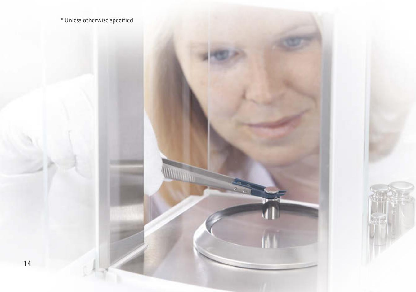
Sartorius Proof Line knob weights of OIML classes F1 and F2 with nominal values of 1 g and higher are made of stainless steel that has a density of 7,950 kg/m<sup>3</sup>. The tolerances of these knob weights comply with OIML R111-1, and they are supplied in high-quality plastic screw-top boxes. Knob weights from 10 g and up feature an adjustment chamber.
