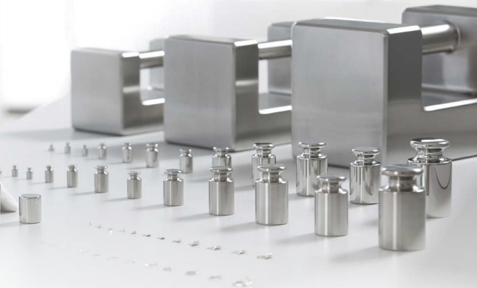
OIML class F1 and F2 cylindrical weights with a lug are made of a special stainless steel that has a density of 7,950 kg/m<sup>3</sup>, and their tolerances comply with OIML R111-1. The weights are delivered in a wooden case suitable for transportation by a pallet mover.
