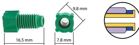
For those systems requiring or preferring flanged connections, use these fiberglass-reinforced fittings with our Easy-Flange flanging tool and polypropylene washers to make a clean connection. The flange on the tubing ensures that the washer never comes in contact with the mobile phase.
