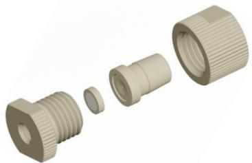
This female-to-female design is made entirely of PEEK, with PEEK-encased titanium or polyethylene filter elements, for biocompatibility and chemical resistance. The design has virtually no hold-up volume and can be used in analytical applications with virtually no band broadening or loss of efficiency.
