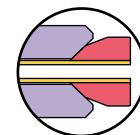
Typically our inverted ferrules are used in these fittings, but the 1/4-28 flat-bottomed details will also accept collapsible ferrule or flanged fittings.
