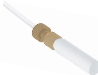
The No-Met polyethylene filter is designed for these applications, with inert polymeric fittings for 1/8" tubing and a 20 µm filter effectively eliminating metal contamination from the fluid path. Use them for IC and biochromatography applications.
