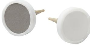
The Last Drop mobile phase filter allows more analyses per batch of mobile phase and helps reduce hazardous waste. The flat filter element sits parallel to the bottom of the reservoir, allowing the Last Drop to filter all but the last 2% of the mobile phase from the reservoir without drawing air into the system. Compare this with conventional cylindrical filters that can begin to draw air into the system when nearly 10% of the solvent remains in the reservoir.
