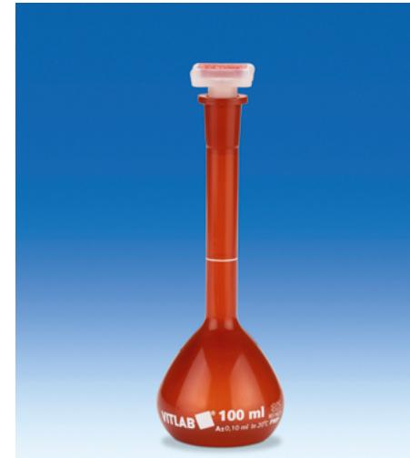
UV-absorbing, highly transparent. For storage of light-sensitive substances.
