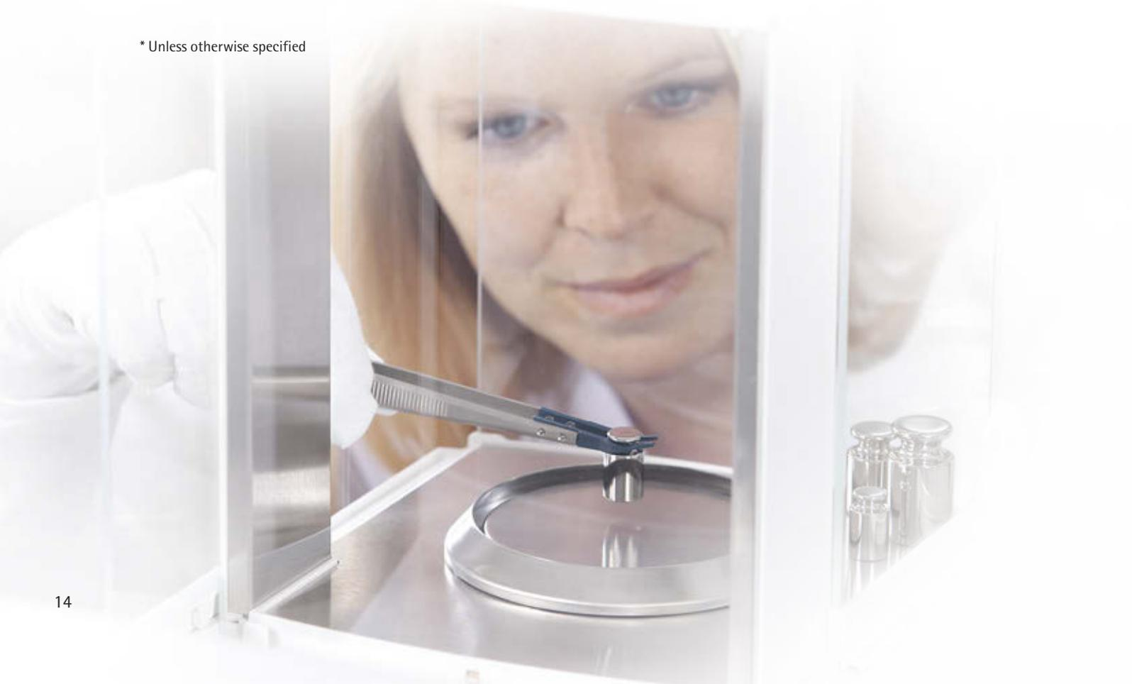
Sartorius Proof Line knob weights of OIML classes F1 and F2 with nominal values of 1 g and higher are made of stainless steel that has a density of 7,950 kg/m<sup>3</sup>. The tolerances of these knob weights comply with OIML R111-1, and they are supplied in high-quality plastic screw-top boxes. Knob weights from 10 g and up feature an adjustment chamber.
