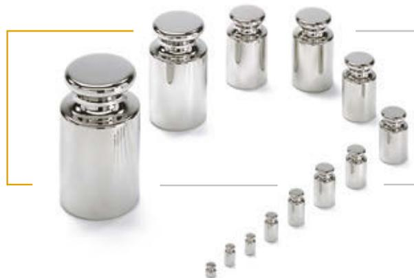
Proof Line OIML class F1 leaf weights ranging from 1 mg to 5 mg are made of aluminum that has a density of 2,650 kg/m<sup>3</sup>; those with nominal values from 10 mg to 500 mg are manufactured from nickel silver that has a density of 8,600 kg/m<sup>3</sup>. Their tolerances comply with OIML R111-1.
