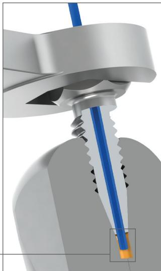
**MarvelX UHPLC fittings** do not depend on ferrules. They seal at the bottom of the port, without complex techniques, which significantly reduces required torque and enables many more connects and disconnects. Furthermore, they are virtually impossible to over-tighten by hand, limiting wear and increasing product life. An enhanced proprietary tip design also ensures zero dead volume (ZDV) and better chromatography results.
